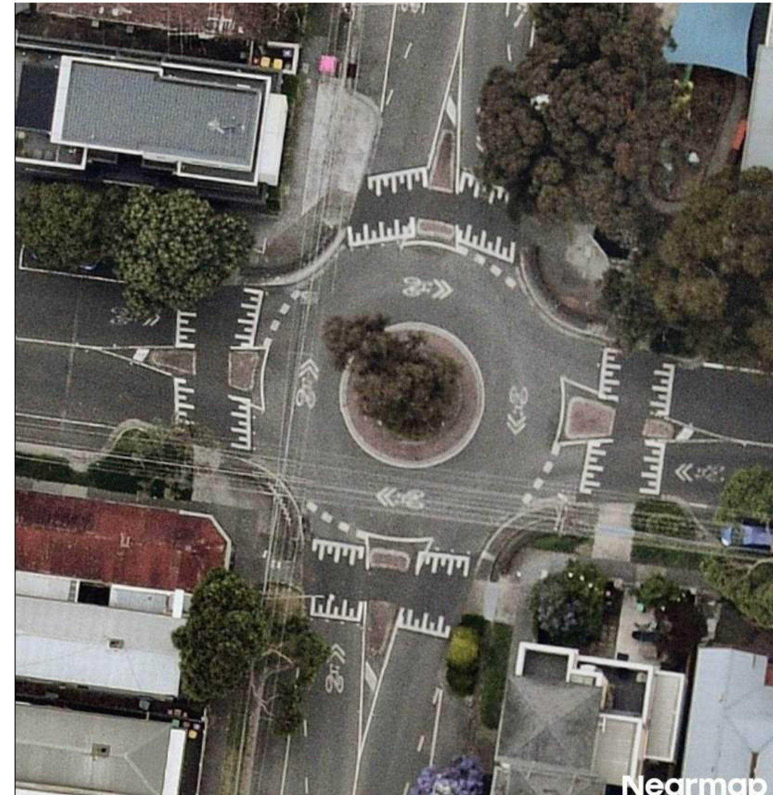
Raised platforms on all legs of roundabout at Kent Street / Gardner Street, Richmond
