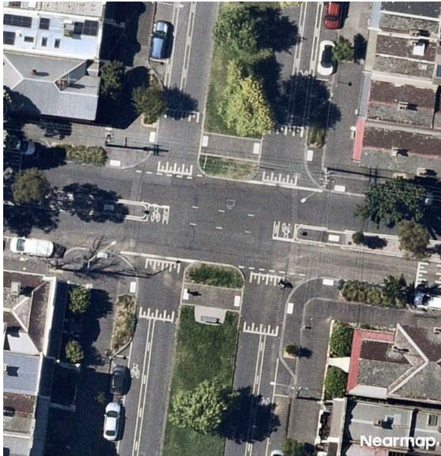
Raised thresholds at Drummond Street / MacPherson Street, Carlton North
